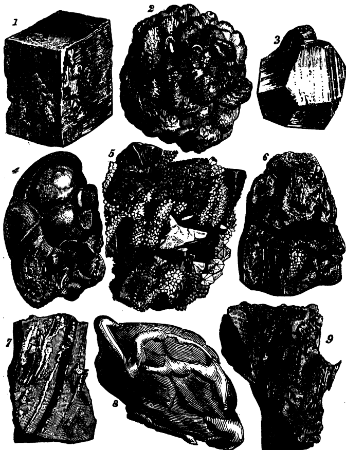
Fig. 115. Series of Specimens, from Mr. Tennant's. 1, 2, 3. Specimens of iron pyrites. 4. Malachite. 5, 6. Copper pyrites. 7, 8, 9. Specimens of rock containing gold.
